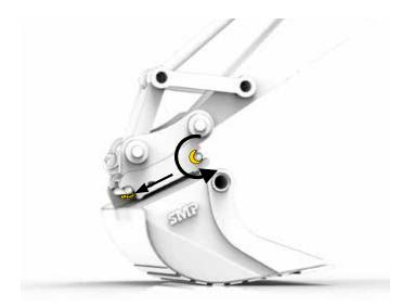
5. Check on the indicators that the quick coupler has locked – both indicators should be "hidden".
